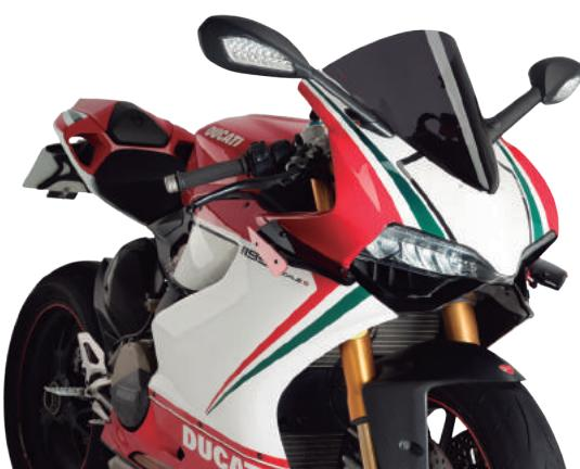
The Downforce that the spoilers generates raises potentially as the speed increases, at 300 km/h we get 3,6 Kg/f.
